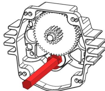
**Step 7:** Place the 48 Tooth Gear (am-0885) on TB Hex Output Shaft with the **flat side touching the 1/2" E-Clip**.
