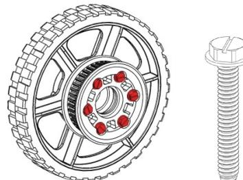
**Step 2:** Using six 10-24 x 1.25" (am-1266) thread forming screws attach the pulley halves to the wheel.
