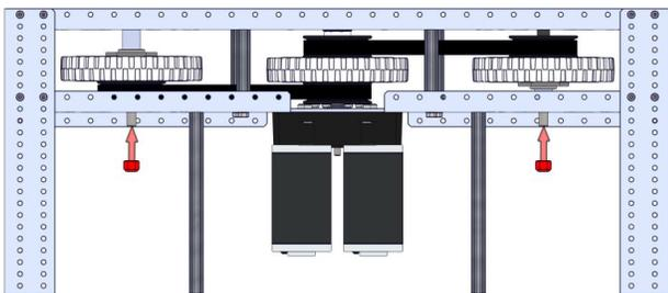
**Step 23:** Add another Outer Wheel Assembly to the other end of the chassis. Loop the belt onto the pulley and insert the assembly between the Inside and Outside Plates. This assembly should have its pulley facing opposite of the first assembly.
