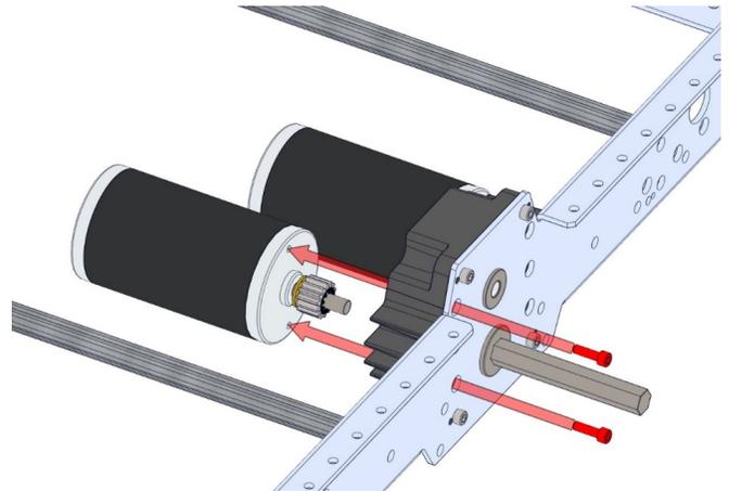
**NOTE:** Each drive gearbox can accept up to 2 motors. Repeat this step for each motor.
