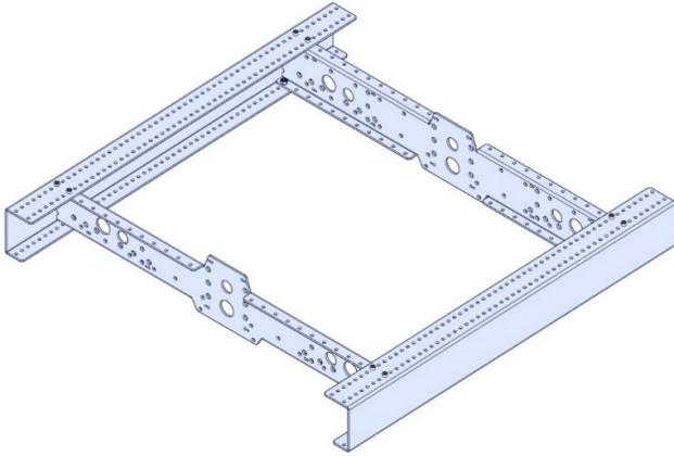
**Step 6:** Attach the two (cut to length) Long Churros between the Inside Plates using four ¼-20 x 0.750" thread forming screws (am-1310). A ½" wrench can be used to hold the churro while tightening.
