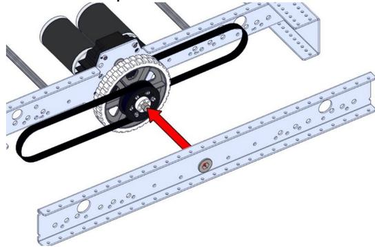
**Step 16:** Secure the Outside Plates to each End Plate using six 10-32 x 0.500 socket head screws (am-1002) and two 10-32 Nylock nuts (am-1042).
