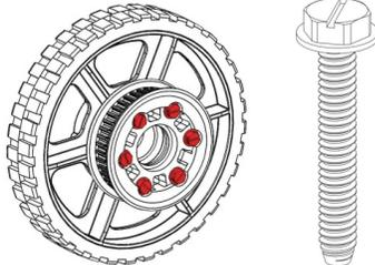
**Step 3:** Press two 1614ZZ bearings (am-0209) into each side of the wheel/pulley.
