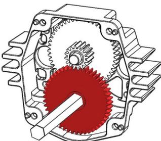
**Step 8:** Apply Red Tacky Grease (am-2768) to all of the gear teeth.
