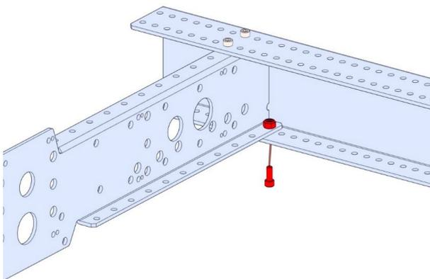
**Step 4:** Repeat steps 2-3 on to attach the other Inside Plate to the End Plate.
