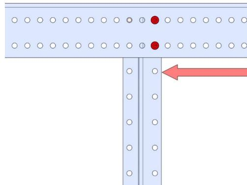
**NOTE:** The top flange of the Inside Plate should point toward the short side of the End Plate
