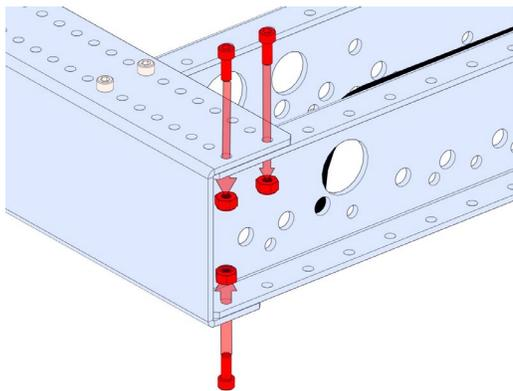
**Step 17:** Attach four 3.375" Churro Standoffs (am-2569) (see below for recommended locations) with 1/4-20 x 0.75" Thread Forming Screws (am-1310) onto each Inside Plate. A 1/2" wrench can be used to hold the churro while tightening. Make sure to loop belts over the churro to ensure the belts have a straight path from axle to axle.
