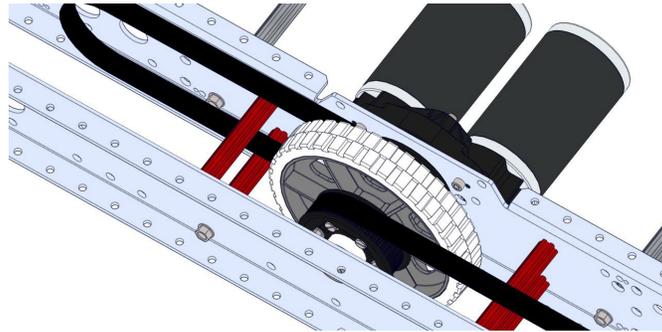
**Step 19:** There are different axle bolt locations for each chassis configuration. Locate the hole to match the chosen belt and frame size.
