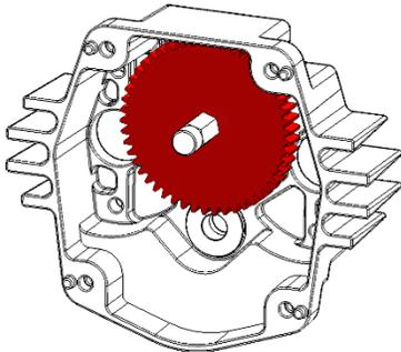
**Step 4:** Place the 16 tooth gear (am-0747) on the TB Small Hex Shaft with **flat side touching the 50 tooth gear**.
