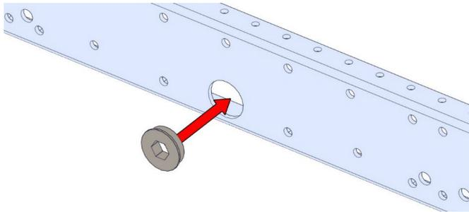
**Step 15:** Place each Outside Plate into the ends of both End Plates with the flanges of the Outside Plate pointing away from the Inside Plate. Ensure the Hex Bearing is aligned to and installed on the Toughbox Mini Hex Output Shaft.
