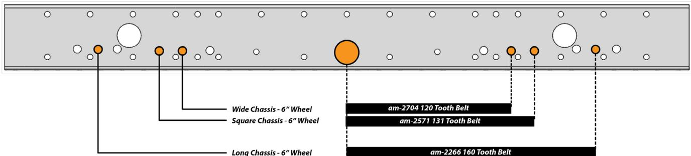
**NOTE:** Axle bolts must be installed from the outside of the chassis. If they are inserted into the Inside Plate first, the included bumper hardware will not fit.
