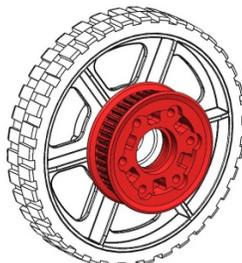
**NOTE:** Tighten the screws in a star pattern to ensure the pulley aligns evenly on the wheel.
