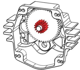
**Step 5:** Tap the 1/2" E-Clip (am-0206) onto the groove on the TB Hex Output Shaft (am-2566a\_K19).
