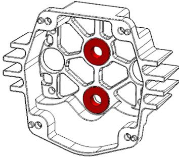
**Step 2:** Insert the TB Small Hex Shaft (am-0152) into the R6ZZ bearing closest to the flat edge of the housing.
