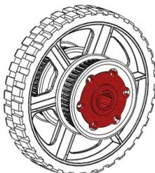
**Step 6:** Add six 10-24 x 1.25" (am-1266) thread forming screws to attach the pulley and hub to the wheel.
