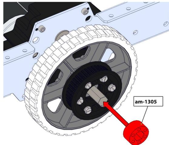
**Step 13:** Select the appropriate belts for your chassis configuration, and loop one belt over each Pulley on each Center Wheel Assembly.
