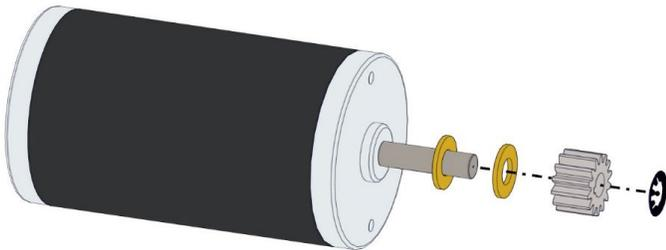
**Step 10:** Line up the CIM motors with the mounting holes in each Toughbox Mini. Secure each motor with gears installed to the Toughbox Mini housing using two 10-32 x 0.625" SHCS w/ Nylon Patch (am-1120).
