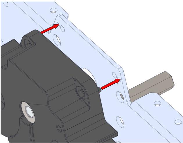
**Step 8:** Attach one Toughbox Mini to each Inside Plate with four 10-32 x 0.75" SHCS (am-1047) and four 10-32 Nylock nuts (am-1042). The nuts will fit into the hex pockets on the Toughbox Mini housing and will hold the nut while tightening.
