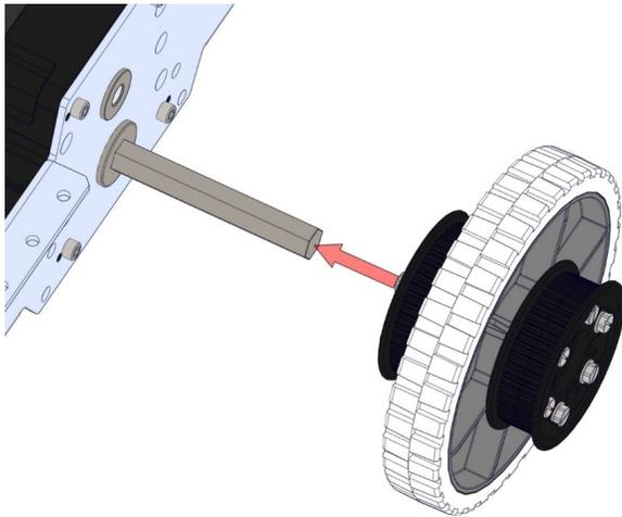
**Step 12:** Place the Hex Spacer (am-1305) onto each Toughbox Mini Hex Output Shaft and press into the round cavity in the pulley. The shaft will help align the spacer hex bore with the wheel hub hex bore.
