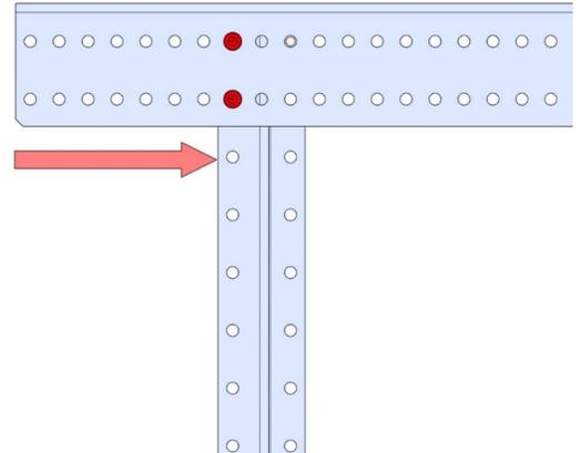
**NOTE:** The top flange of the Inside Plate should point toward the short side of the End Plate
