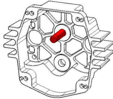
**Step 3:** Place the 50 tooth gear (am-0149) on the TB Small Hex Shaft with the **small round boss touching the bearing** and the flat side of the gear facing away from the housing.
