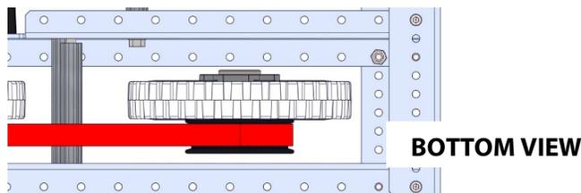
**NOTE:** The belts should be parallel to the side plates.
