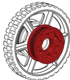
**Step 5:** Insert one 500EX Hex Hub (am-2568) into the pulley on one side of the wheel.
