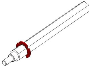
**Step 6:** Insert the small end of the TB Hex Output Shaft (am-2566a\_K19) into the other R6ZZ bearing.
