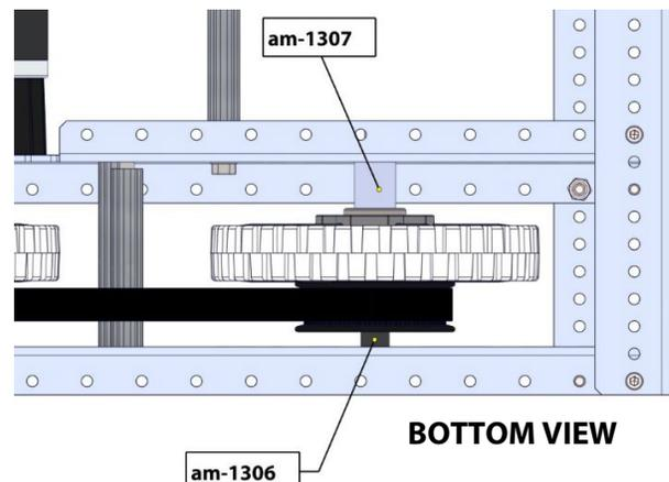
**Step 22:** There are different axle bolt locations for each chassis configuration. Slide a  $\frac{3}{8}$ " axle bolt (am-1297) through the spacers and wheel assembly, with the head of the bolt pointing away from the chassis.
